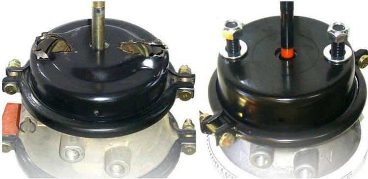
The larger the contact area between the mounting face of the springbrake and the axle bracket, the further away the 'fulcrum point', and the lower the tensile stresses imposed on the mounting studs.
